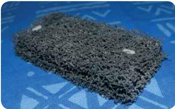
Figure 2. A small sample of novel invertebrate enhancing artificial substrate pad material. Large sections of this material will be attached to the exterior of select experimental ARs.
