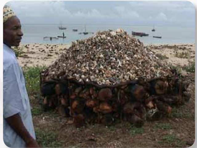
Pile of coral ready to be burnt to make concrete.
